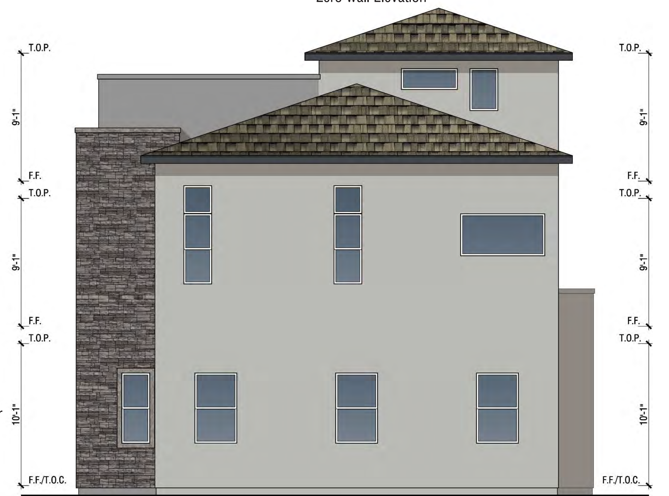
Right Side yard Elevation
